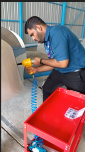
Figure 4: The riveting process using Portable Rivet Lander Machine at UniCAM Hangar
