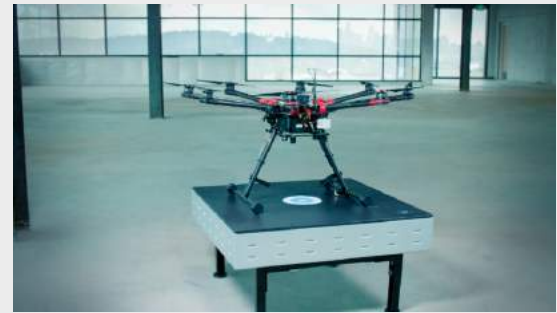
Wireless charging system that WiBotic develops
